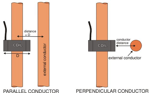
*Parallel conductor:* This is a common configuration for example three phase conductors in the same enclosure. Under these conditions the pick-up ratio is less than 1%. The pick-up ratio reduces for larger values of distance and is roughly proportional to  $1/(\text{distance})$ .
