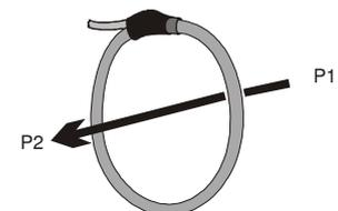
**1.4 Insulation:** Unless otherwise specified it should NOT be assumed that the coils are insulated against high voltages. Additional insulation should be used with conductors carrying dangerous voltages.
