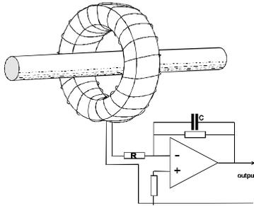
not influenced significantly if the conductor is positioned 'off-centre'. The design also ensures that the influence from currents and magnetic fields external to the coil is minimal.
